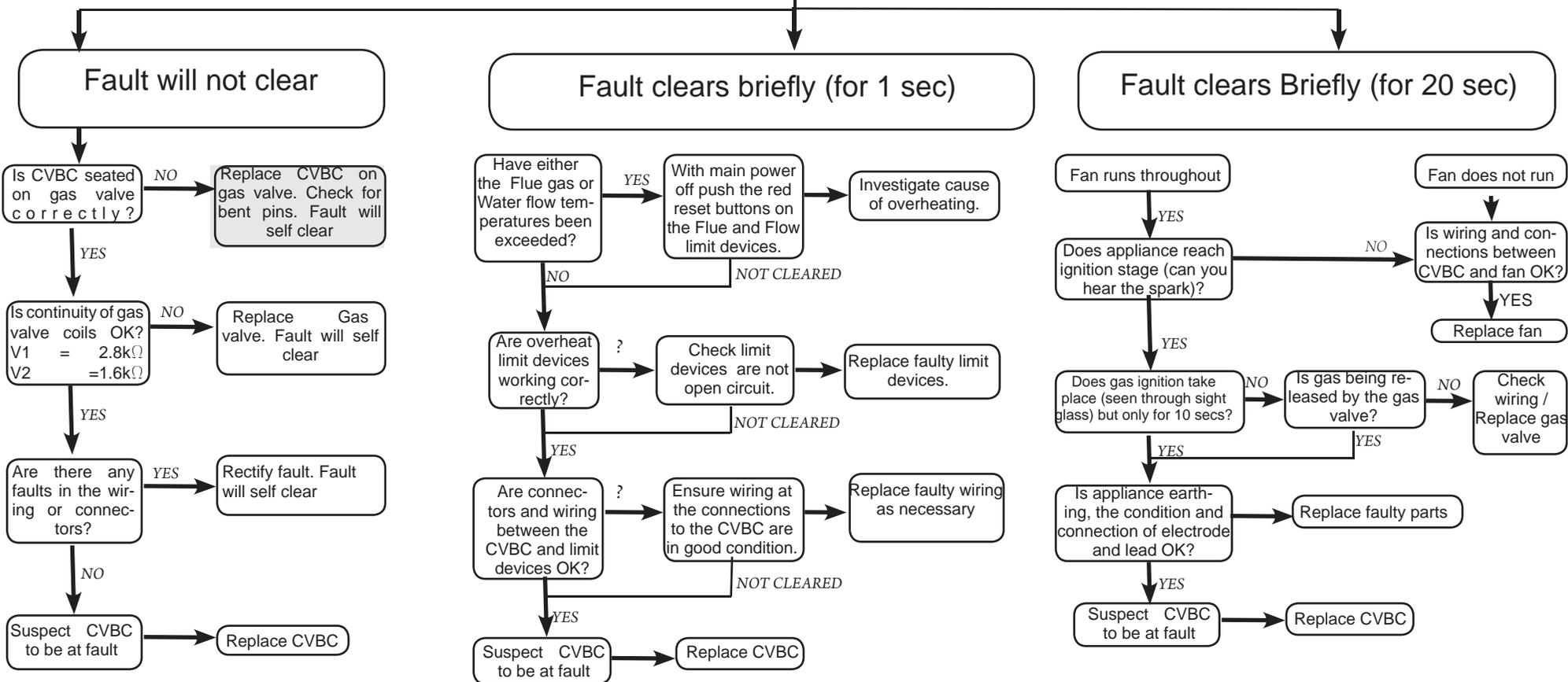
**NB - A fault involving the Gas valve circuit will occur even if there is no heating demand. Reset appliance when there is no heat demand to identify a fault of this nature. Once corrected, there is no need to use the reset button, as the fault will self clear.**
